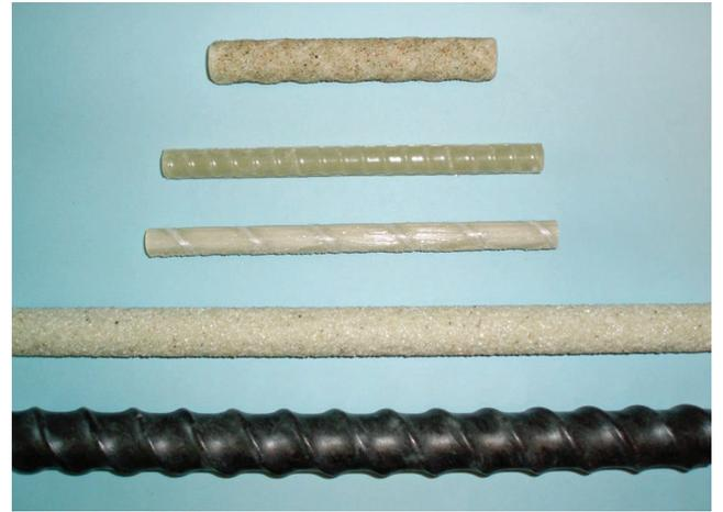
Fig. 1.1—Examples of FRP reinforcing bars.
